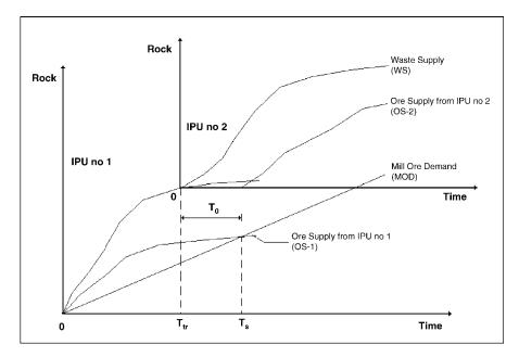
Fig. 2. Determining the time of transition of the mining operations from one IPU to another and related notation (please refer to the text for explanations).
