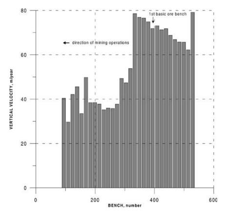
Fig. 7. Vertical velocity versus bench in IPU no. 5.
