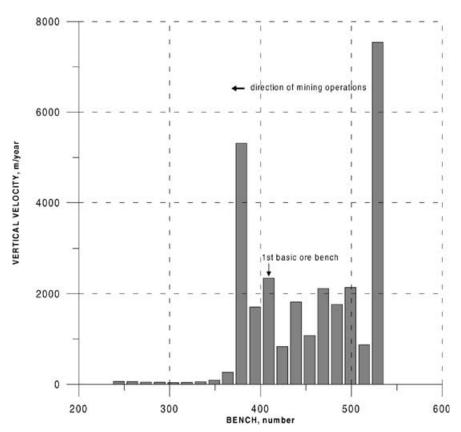
Fig. 4. Vertical velocity versus bench in IPU no. 2.
