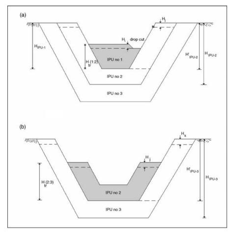
Fig. 3. Schematic representation of the transition from (a) IPU no. 1 to IPU no. 2; and (b) IPU no. 2 to IPU no. 3 (please refer to the text for discussion).
