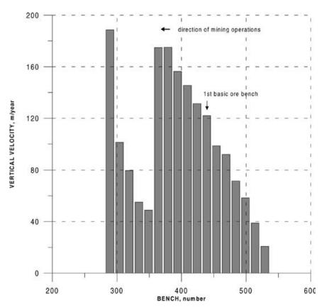
Fig. 6. Vertical velocity versus bench in IPU no. 4.
