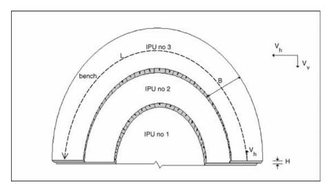
Fig. 1. Schematic representation of an open pit mine with three IPUs showing the geometric characteristics of a working bench; please refer to the text for details.
