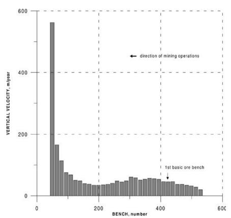
Fig. 8. Vertical velocity versus bench in IPU no. 6.
